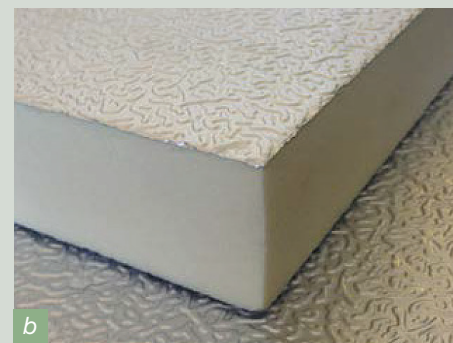
Figure 3: a) Schematic Illustration of the continuous insulation concept for a timber frame wall, b) PIR board insulation with foil facers (photo courtesy of Pirmax Pty Ltd).
